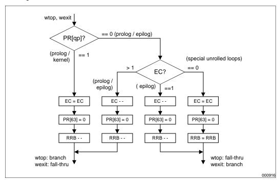
Figure 11-2. wtop and wexit Execution Flow
