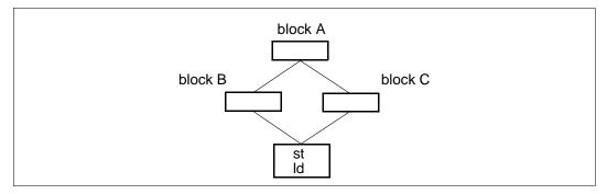
If the compiler or programmer advanced the load up to block B from its original non-speculative position, all speculative code would need to be duplicated in both blocks B and C. This duplicated code might be able to occupy NOP slots that already exist. But if space for the code is not already available, it might be preferable to advance the load to block A since only one copy would be required in this case.
