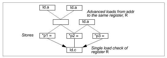
A single check in the lowermost block shown for all of the advanced loads is correct if both of these conditions are met:
