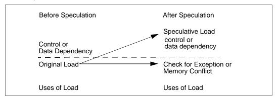
The check detects a deferred exception or a conflict with an intervening store and provides a mechanism to recover from failed speculation. With this support, speculative loads and their uses can be scheduled earlier than non-speculative instructions. As a result, the memory latencies of these loads can be hidden more easily than for non-speculative loads.
