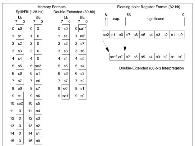
Figure 5-10. Spill/Fill and Double-extended (80-bit) Floating-point Memory Formats
